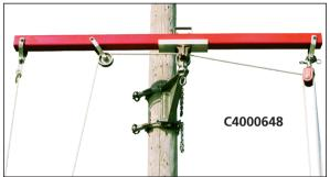
The gin beam can be rotated in a half circle, swinging the load away from underbuild obstructions. Rocker-action of the beam, up to 60°, controls distance of the load from the pole.
